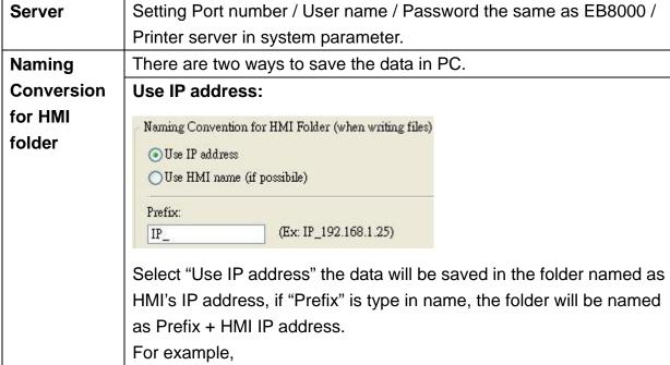
The prefix is IP\_ and HMI IP address is 192.168.1.104, the folder in C:\EB8000 as below (IP\_192.168.1.104)
