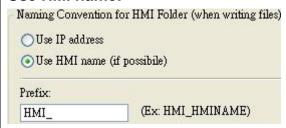
Select "Use HMI name" the data will be saved in the folder name as HMI name (LW9032~LW9039 total 8 word), if "Prefix" is type in name, the folder will be named as Prefix + HMI name.
